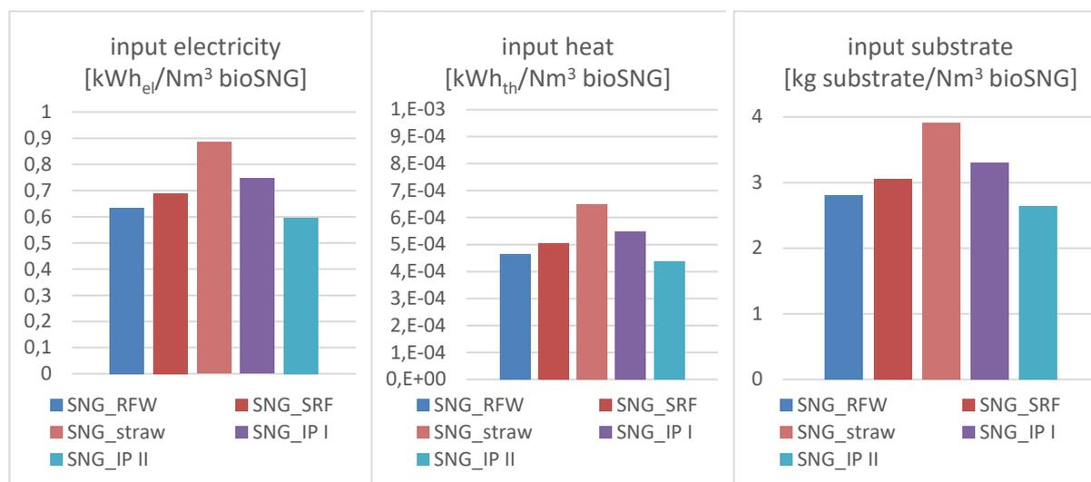
Figure 11: BioSNG - input values gasification and upgrading
