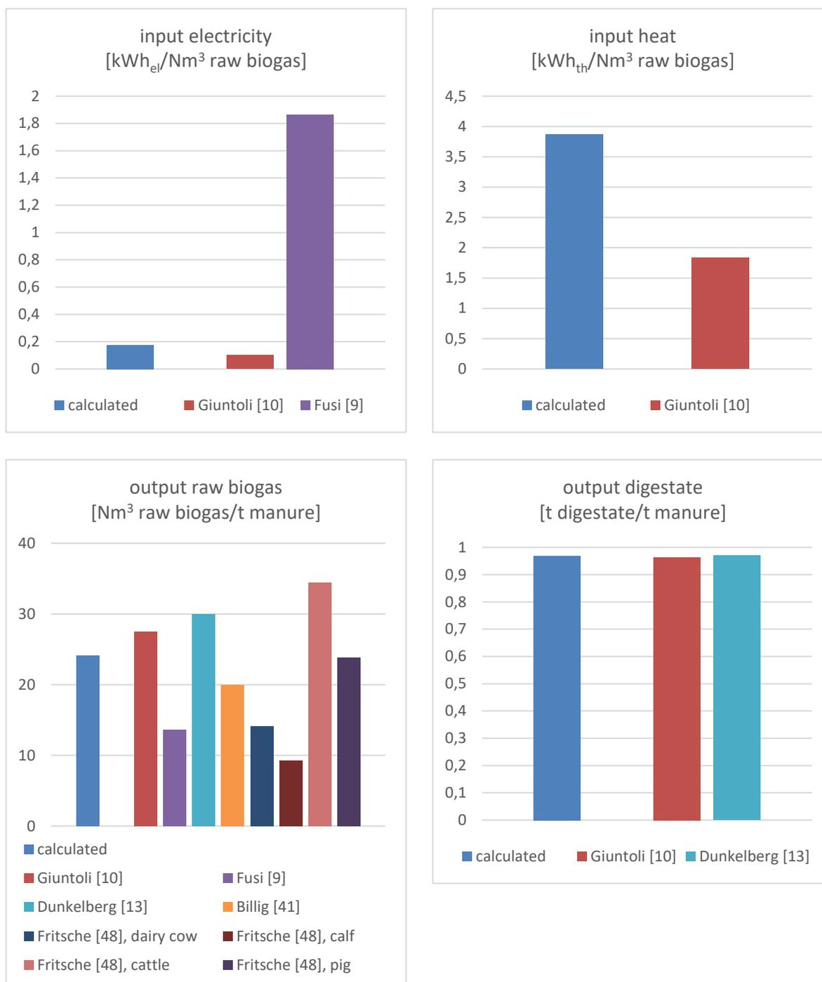
Figure 3: Anaerobic digestion of manure: Comparison of calculated values with literature data
