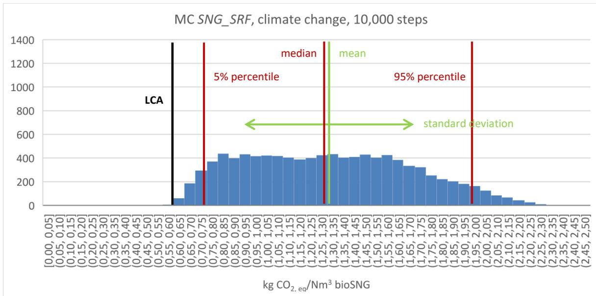
Figure 15: Results Monte Carlo simulation *SNG\_SRF*, climate change, 10,000 simulation steps
