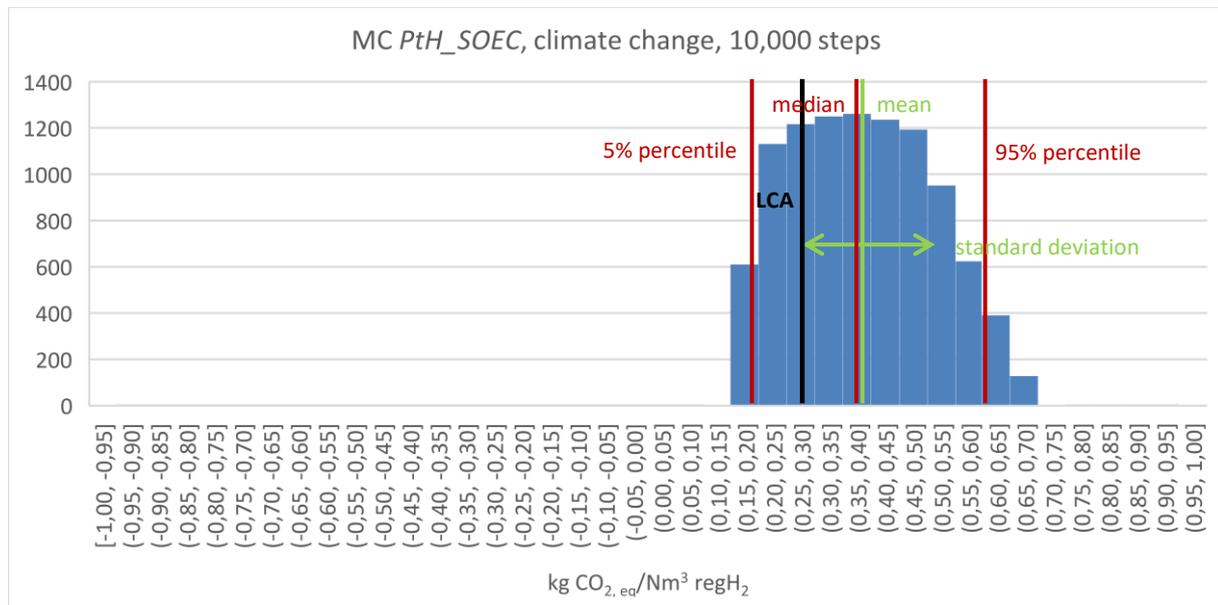
Figure 24: Results Monte Carlo simulation *PtH\_SOEC*, climate change, 10,000 simulation steps
