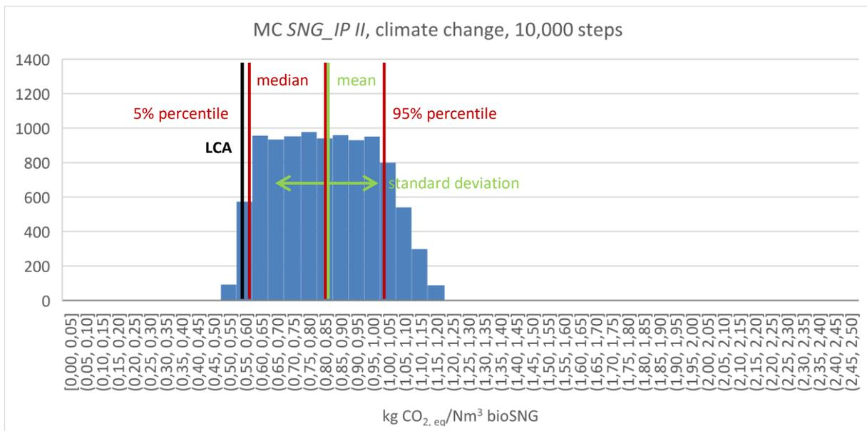
Figure 18: Results Monte Carlo simulation *SNG\_IP II*, climate change, 10,000 simulation steps
